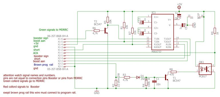
The red wire from the booster has also to be connected to the other track of the program rail
